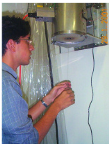
Figure 7. Alex Argyros draws one of our first plastic fibres by hand using a furnace borrowed from another group. Image: J. Zagari
